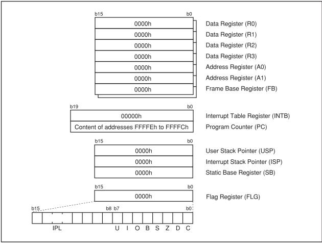
Figure 5.3 CPU Register Status After Reset
